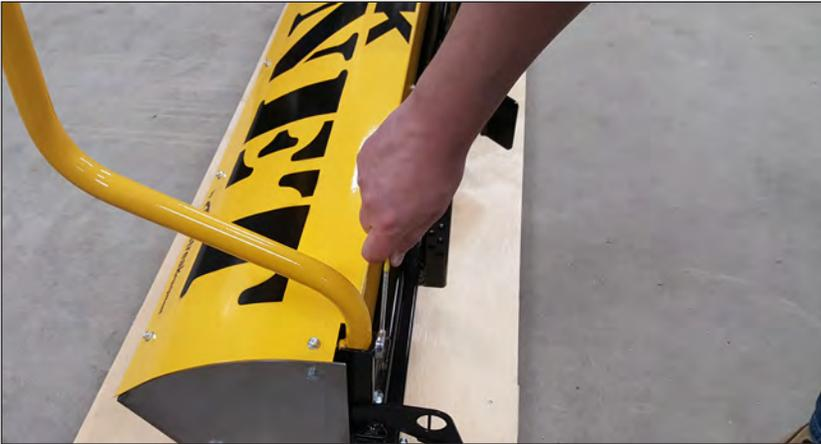
Remove the handle from the pallet and un-wrap. Remove both bolts and washers from the end of the handle. Place handle with welded nuts facing inward toward the lid in the position shown in the picture.
