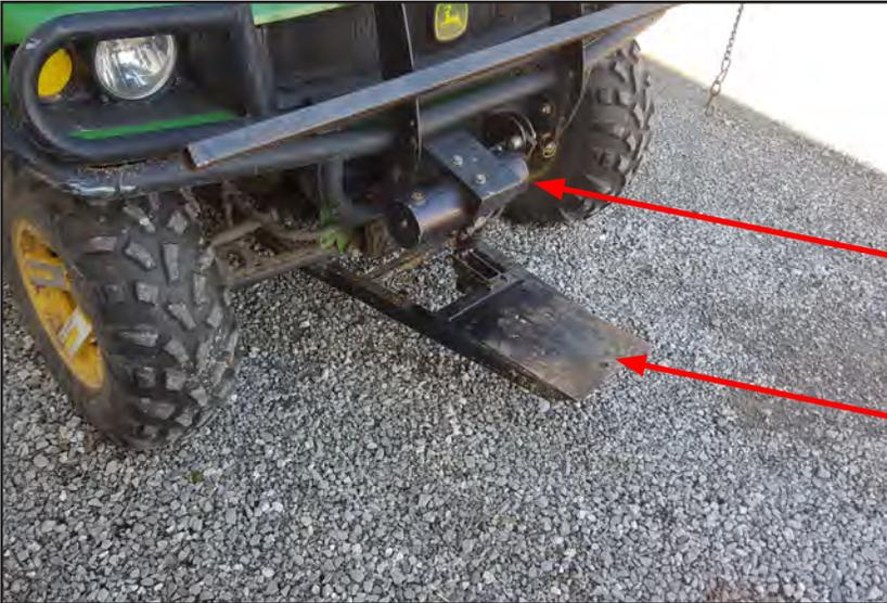
Remove Snow Plow from Push frame of UTV to prepare for Mounting Yak Quick Hitch
