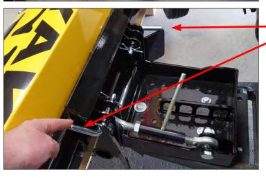
Bent Pins (with clips)
