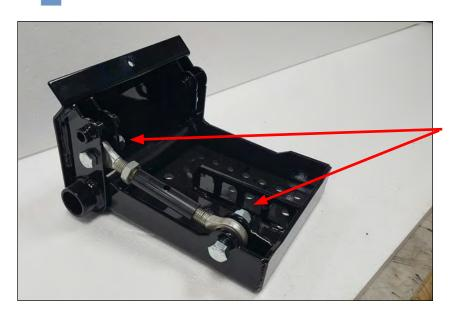
Attach both sides of the Top Link to the Quick Hitch using the 2-5/8" x 2 1/4" Bolts and 2-5/8" Nyloc Nuts.
