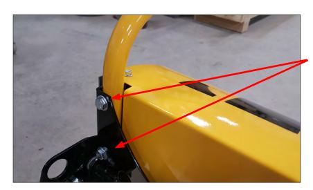
Fully tighten both bolts using a 9/16 wrench.
