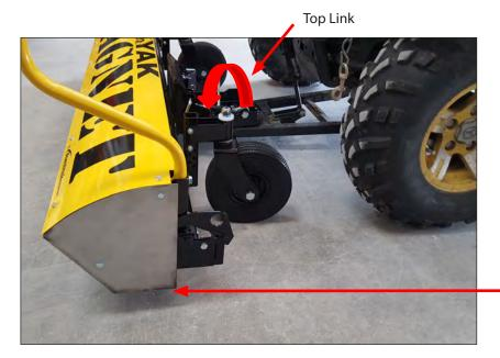
Adjust Top Link with the adjuster rod until the bottom of the magnet is level with the ground.
