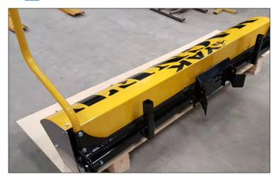
Slide the magnet so the back of the sweeper is at the edge of the pallet as shown.
