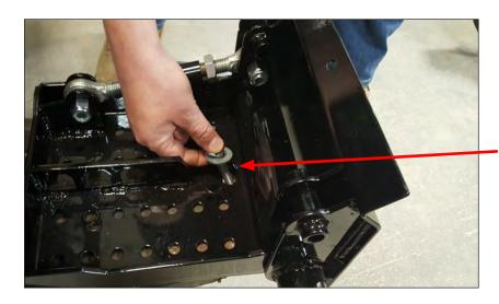
Install the ½" x 2" bolt in the Plow Pivot Hole location. Use a washer on top and bottom and thread on the ½" Nyloc Nut underneath. Do Not Fully Tighten Yet.
