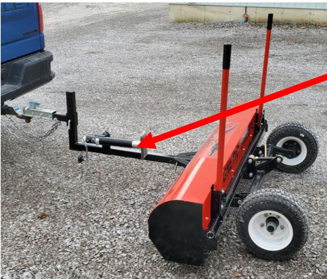
The tongue of the sweeper should be as level as possible. This can be adjusted by changing the position of the coupler on the trailer tongue or the ball mount on the tow vehicle.
