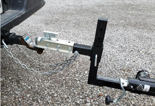
Connect the sweeper to the tow vehicle with the 2" ball coupler and safety chains. You must use a 2" Trailer ball, unless you purchased an optional Pintle Ring.
