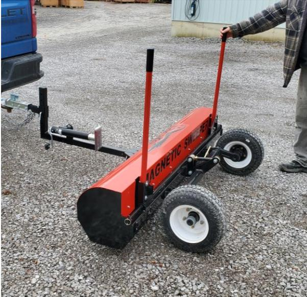
Return debris release handle to upright position and continue sweeping to collect more metal debris.
