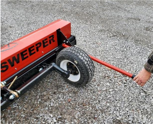
To clean debris off of the magnet. Stop the tow vehicle.
