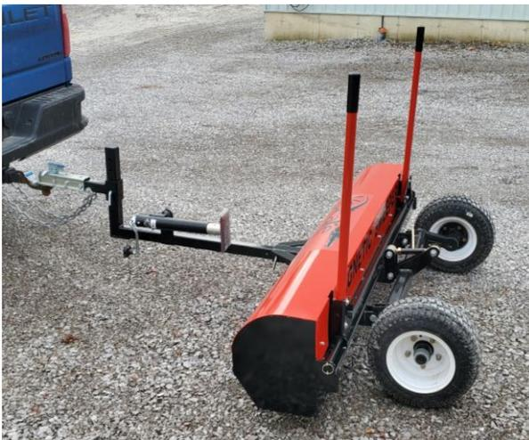
Drive around with magnet and collect metal debris.
