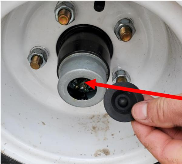
Remove rubber cap and using a grease gun apply wheel bearing grease to the grease nipple in each wheel hub once per year.
