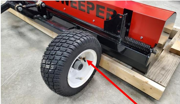
Install both wheels with valve stem facing out.
