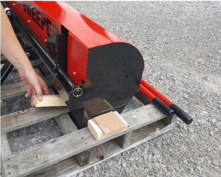
Remove the wooden blocks that are attached to the pallet from the ends and back of the sweeper.
