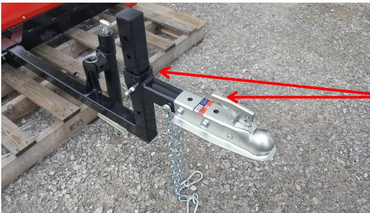
Install Coupler Assembly and insert a Bent Pin and clip.
