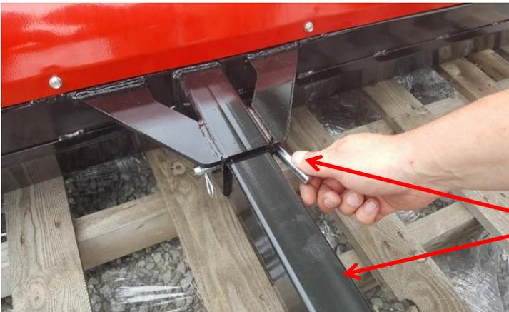
Install Steel Tongue and insert a Bent Pin and clip.
