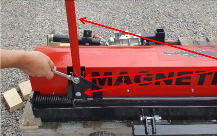
Install Release Handles on each end of the sweeper and tighten using a 9/16 wrench.
