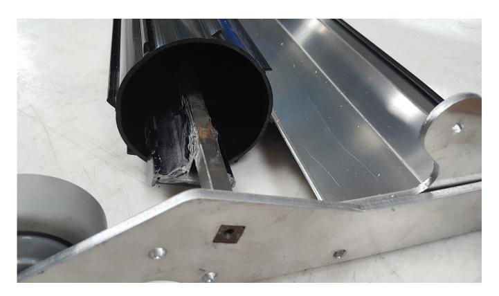
Theta - Black finned PVC Replacement Drum Assembly Instructions: Install the new Finned PVC Drum so the orientation of the Fins on the drum and the Magnet Assembly are exactly as the shown in the photo. (Note: Some magnetic sweeper parts have been removed in the photo so the orientation of the Finned Drum and Magnet Assembly can be easily seen.)
