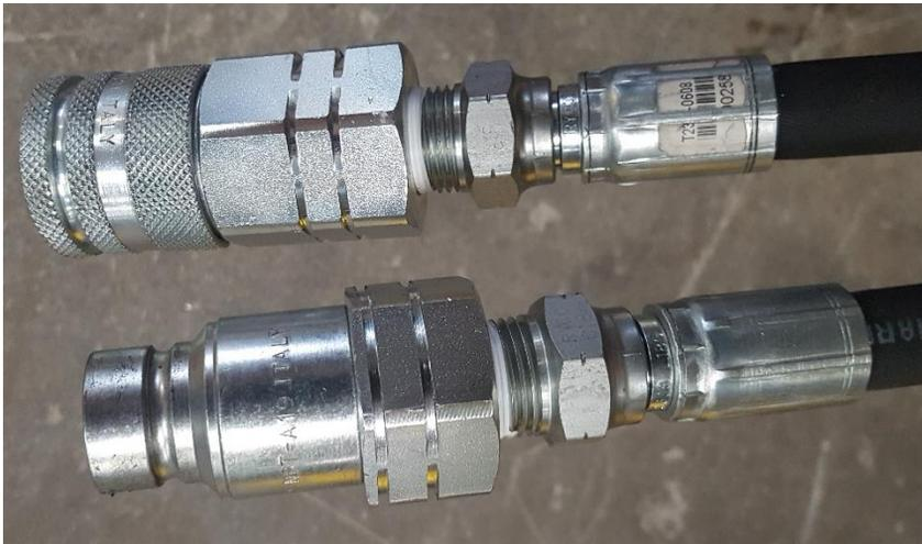
Connect the hydraulic hoses on your Sunda to the auxiliary supply couplers located on your skid steer loader lift arm.
