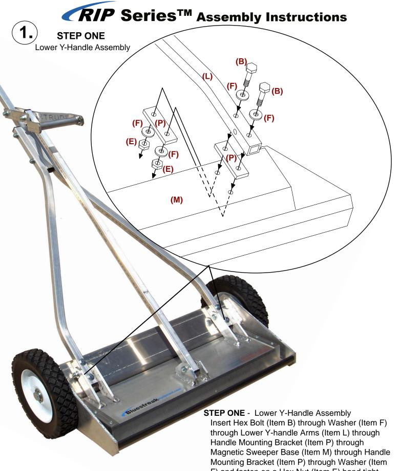
Magnetic Sweeper Base (Item M) through Handle Mounting Bracket (Item P) through Washer (Item F) and fasten on a Hex Nut (Item E) hand tight only. Repeat this step for both holes on each side of the magnetic sweeper. Do not tighten bolts used in this step until completing step 2.
