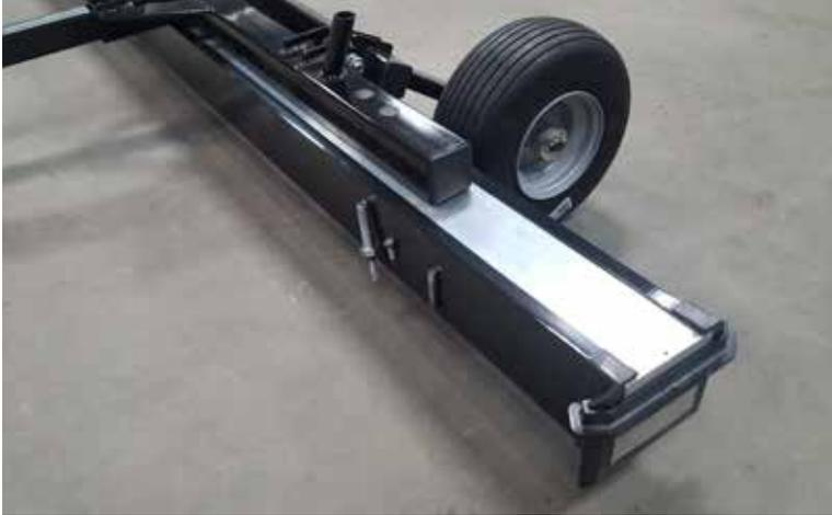
Use sweeper to pick up metal debris.
