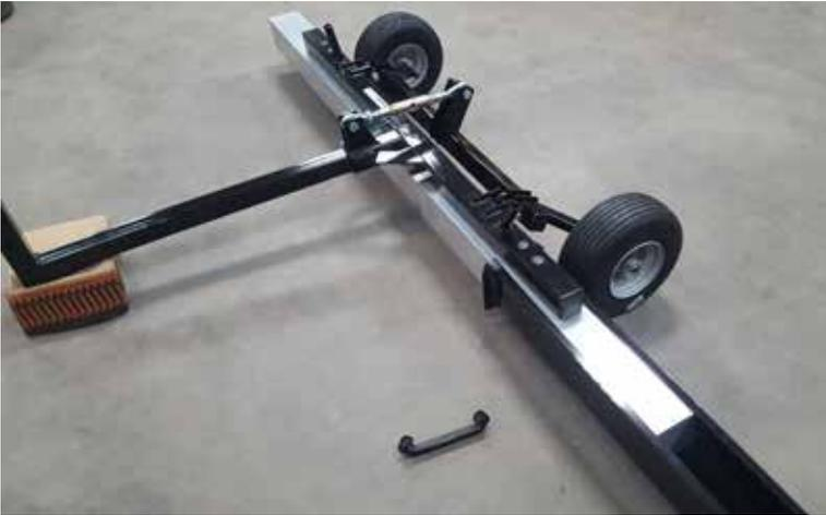
Make sure magnet housing (Square Aluminum Tube) is clean before installation. Remove one of the Plastic Stoppers from one end of the sleeve and slide sleeve onto aluminum housing.
