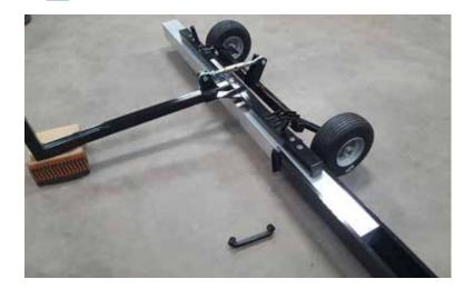
Make sure magnet housing (Square Aluminum Tube) is clean before installation. Remove one of the Plastic Stoppers from one end of the sleeve and slide sleeve onto aluminum housing.
