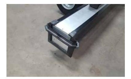
Re-install previously removed Plastic Stopper.
