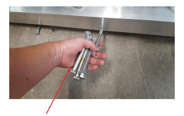
Stop and clean the magnet off before it gets completely covered with debris as magnet performance will decline as more debris is accumulated on it.
