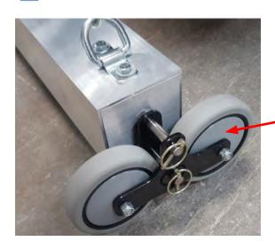
Correct orientation of wheel assembly.
