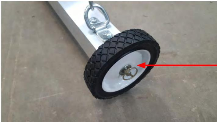
Insert a Lynch Pin (Part C) into hole on the wheel bolt.
