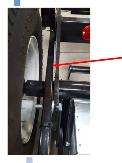
Install Fender Assembly over Bolts.
