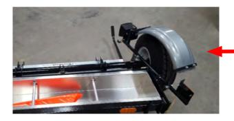
Set the fender assembly on the wheel.
