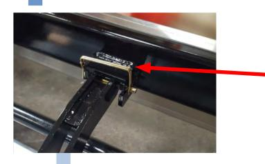
Secure the magnet in the sweeping position by inserting the spring clip (removed in Step #1) into the slot as shown.
