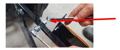
Remove the bolts (x2) washers (x6) and nuts (x2) from the fender assembly.
