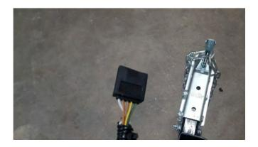
The Lights and Fenders Package comes standard with a 12 volt, 4 flat wire plug.
