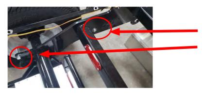
Insert the Bolts from the inside of the frame of the Piranha Sweeper.
