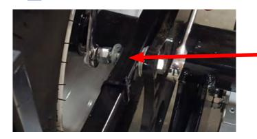
Install 1 washer and 1 Nut on each Bolt and tighten firmly with 9/16" wrenches.
