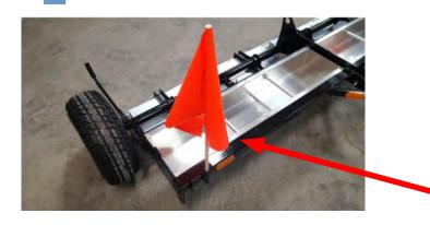
Install the Flag (Item B) in the pocket on each side of the magnetic sweeper.
