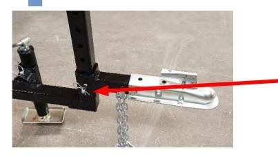
Install the Coupler Assembly (Item E) over the Steel Tongue (Item A) and secure with a Bent Pin and clip (Item D).
