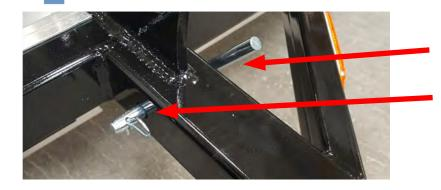
Install a Bent Pin and clip (Item D). Ensure the pin goes though the hole in the tongue by pulling the tongue in and out to make sure the pin secures the tongue from being removed.
