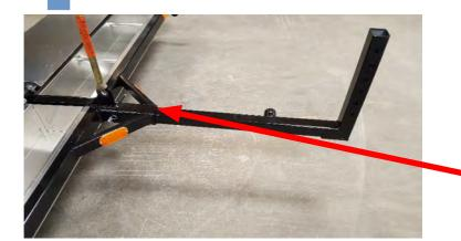
Using the forklift lower the magnetic sweeper until the wheels contact the ground.
