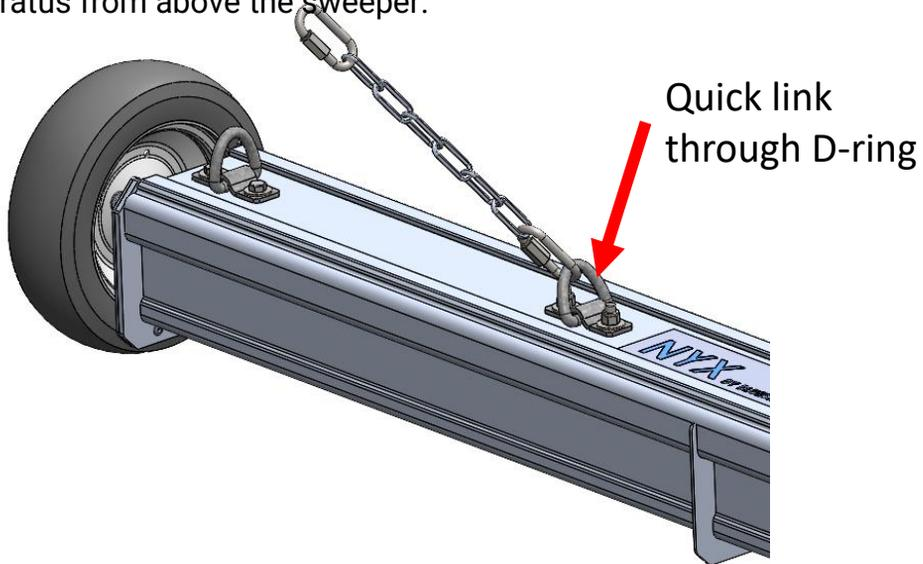
Locate the 4 longer chain assemblies. Unscrew one quick link and hook it through one of the D-rings in the center. Repeat so that there are 2 assemblies on each center D-ring.
