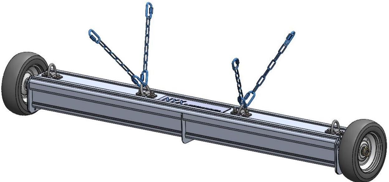
Attach the remaining three chain assemblies in the locations shown. Retighten all quick links in place once looped through the holes.
