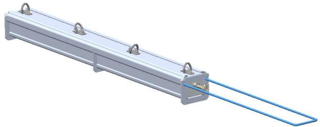
**Step5b:** Pull the handle out until it bottoms out on the quick clean off flange.
