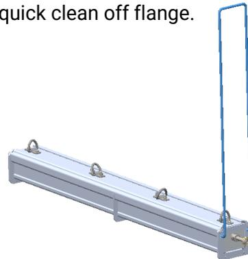
**Step5d:** Remove the handle. To reinstall, you must have the handle perpendicular to the sleeve so that it goes inside the grooves easily
