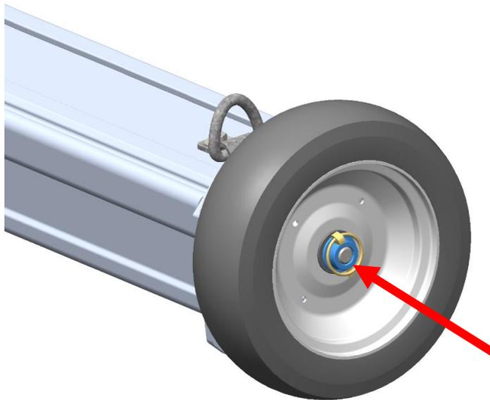
Re-install the retainer and the 3/16" lynch pin. The holes in the retainer and wheel bolt should be aligned. Note: There is a bit of lateral play in the wheel when installed, this was designed this way for optimum rolling behaviour. Repeat for both sides.
