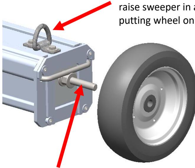
Install the flat proof wheel on the wheel bolt. Note the orientation of the wheel as shown. The bump wheels will not work as intended if the wheel is installed the other way around. Repeat for both sides.
