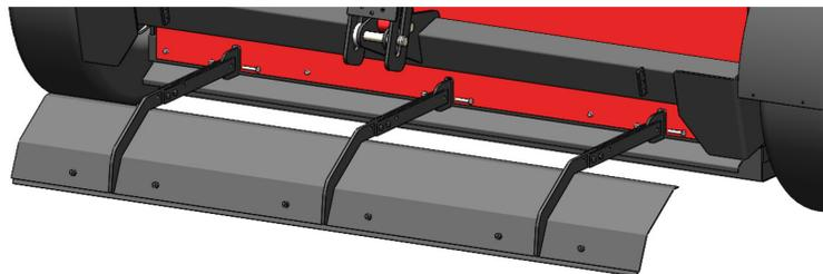
3/8" x 1.75" - Grader link 1 - 3/8" washer - Mounting tab - 3/8" washer - Grader link 2 - 3/8" nut
