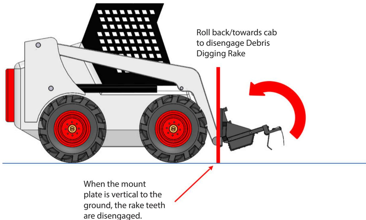
To operate the Lynx without engaging the optional Debris Digging Rake, roll the attachment plate on your machine back so the mount plate of the Lynx is vertical to the ground. When the mount plate is vertical the teeth of the Debris Digging Rake will sit higher than the bottom of the Lynx debris pan. Rolling the attachment back will NOT impact the magnets strength, so a recommended sweeping height of 2"- 5" above the ground should still be maintained.
