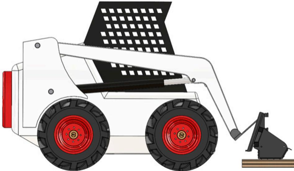
Verify that the coupler plate is free from dirt / debris and metal debris from previous uses. When clear, move the skid steer to proximity of coupler plate. Tilt skid steer coupler forward to align coupling point with the upper part on the attachment plate and raise the coupler slightly.
