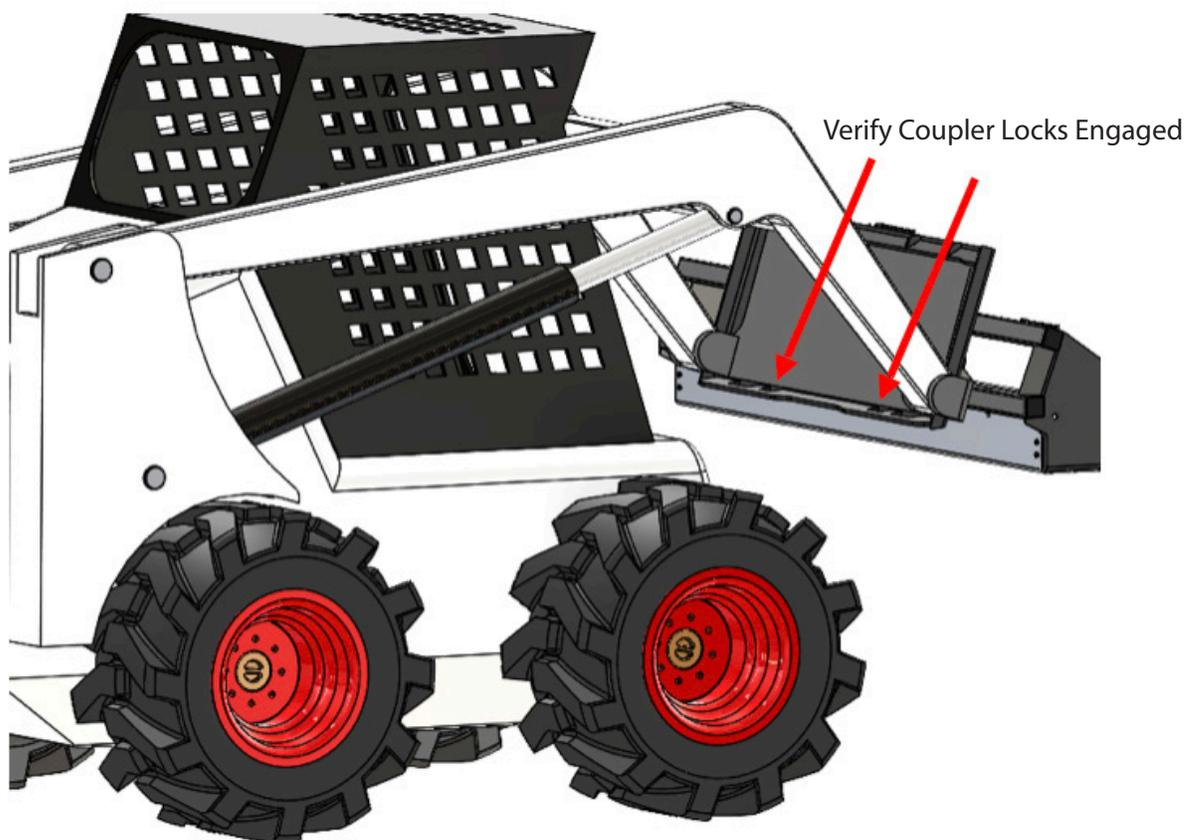
Before operating the attachment, always visually inspect and verify that the coupler lock pins are fully engaged through the latch slots on the attachment plate.
