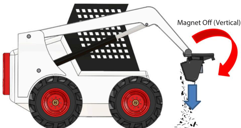
Once the Lynx is elevated pivot the magnet forward into the shown vertical position and the collected debris will fall off the bottom.
