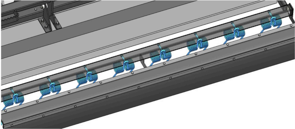
Install the eight steel springs (rake teeth), each with one 3/8" x 3.5" bolt, two 3/8" washers, one 1/2" washer, and one nyloc nut in the order shown below.
