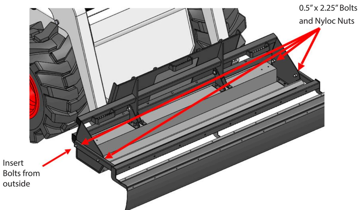
With two people, lift the debris digging rake so that the holes in the arms line up with the holes in the side plates. Insert the four included 0.5" x 2.25" bolts from the outside and secure with included Nyloc Nuts.
