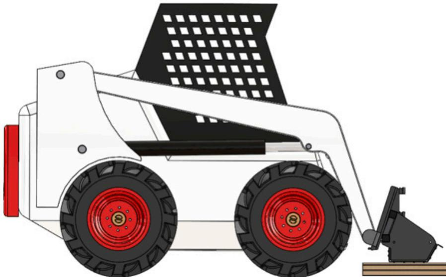
When the top edge of the coupler is seated in the top part of the coupler plate, roll the skid steer tilt function back until the attaching plate is flat against the skid steer coupler. Lock down the coupler levers. Note: If your skid steer is equipped with a hydraulically operated coupler, activate the coupler lock at this time.
