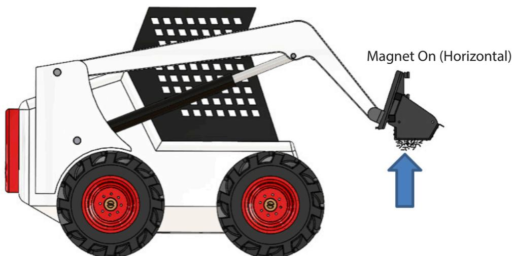
Lift the Lynx using the lift arms are least 48" off the ground, or alternatively you can lift the sweeper even higher if releasing debris into a bin.
