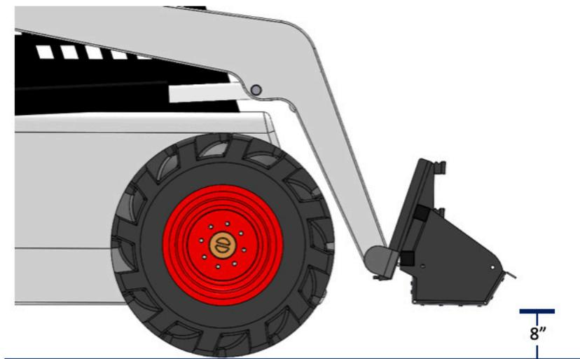
Apply the parking brake to the machine and lift the sweeper a MINIMUM of 8 inches off the ground for installation of the accessory Debris Digging Rake.
