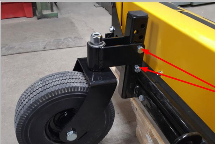
Select desired wheel height by selecting the hole height of the casters.
