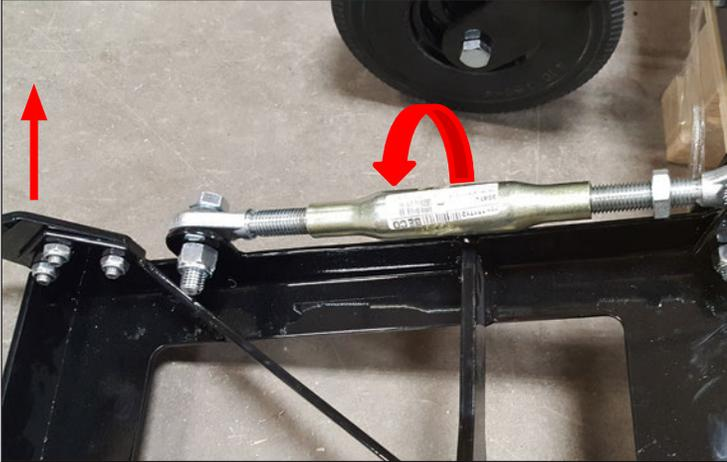
Turn the Top Link to raise the Steel Back Frame to the approximate height required to insert parts B and C into the Provantage Plow Mount bracket that is attached on the ATV.
