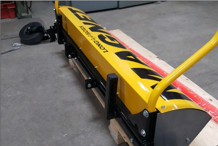
Using the handles slide the magnet so the back of the sweeper is at the edge of the pallet as shown.
