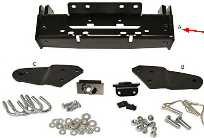
Install Part A of the Warn Provantage ATV Plow System as per instructions in your WARN plow mount kit.
