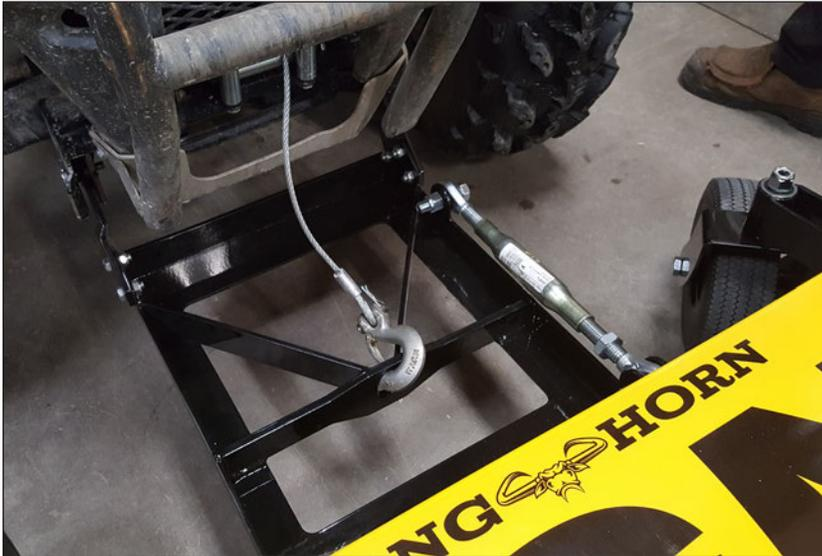
Let out the winch cable on the ATV and hook it into the center hole of the Steel Back Frame.
