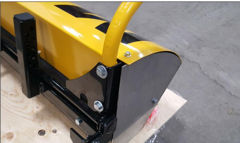
Re-Install bolts with washers as shown.
