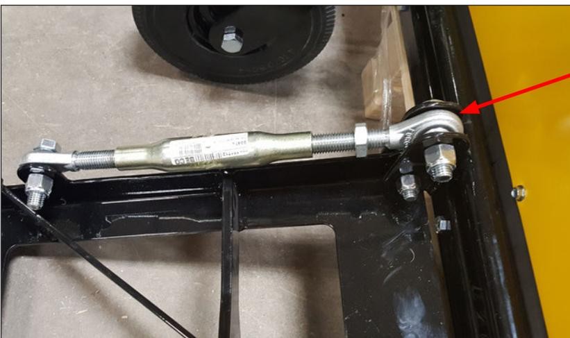
Attach the Top Link to the steel front frame using the 5/8 bolt and nyloc nut that was installed in the Top Link.
