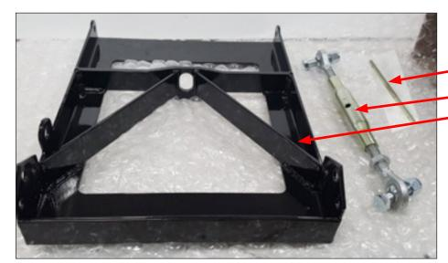
Unpack the Pallet Remove items from the pallet including: 1- Top Link Adjuster 2 - Top Link with bolts
