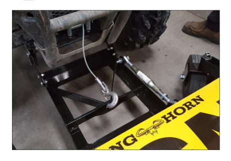
Let out the winch cable on the ATV and hook it into the center hole of the Steel Back Frame.
