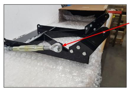
Attach one side of the Top Link to one side of the Steel Back Frame using the bolt that came with the Top Link.
