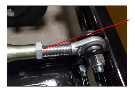
Be sure to tighten the nut on the Top Link firmly when you are finished adjusting to prevent it from coming out of adjustment.
