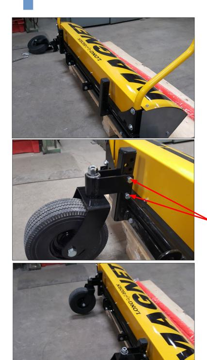
Using the handles slide the magnet so the back of the sweeper is at the edge of the pallet as shown.
