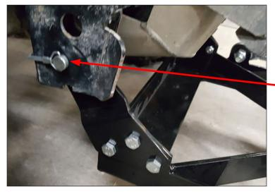
Turn the Top Link to raise the Steel Back Frame to the approximate height required to insert parts B and C into the Provantage Plow Mount bracket that is attached on the ATV.
