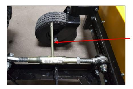
With the Longhorn lowered and resting on the casters, adjust Top Link with the Top Link Adjuster Rod until the bottom of the magnet is level with the ground.
