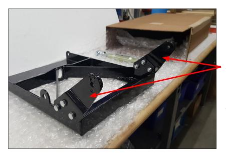
Attach Part B and C of the Plow Mount System to the outside of the Steel Back Frame on each side as shown. To attach Part B and C use the fasteners provided with the Plow Mount Kit.
