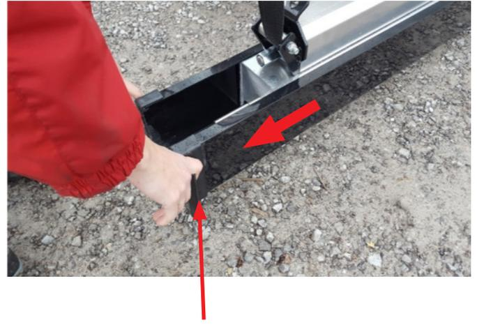
2. Remove the plastic clips on both ends then slide the Quick Clean Off Sleeve off of the aluminum housing.
