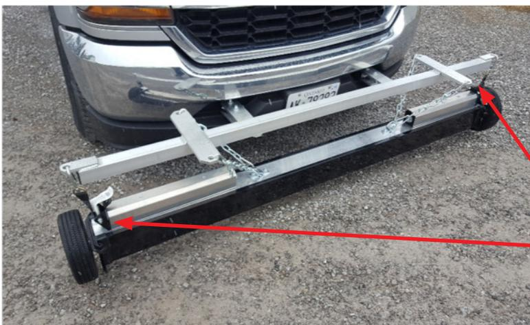
2 Adjuster Straps should be tight and secure.
