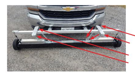
When the magnet is at the set sweeping height the 4 long hanging chains attached to the Magnet D-Rings should be tight and secure and set at an angle from the mounting bracket to the magnet.
