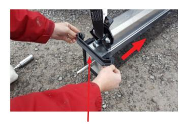
3. Once the magnet is clean, slide the Sleeve back on and re-install the plastic clips on each end.
