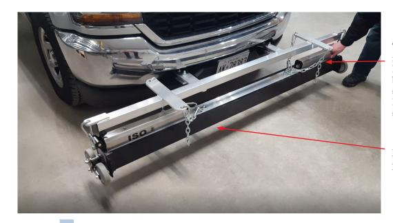
The ISO raised and ready for high speed travel. The hanging chains may be loose but keep them in place for safety. The Adjuster Straps however will be tight and secure.
