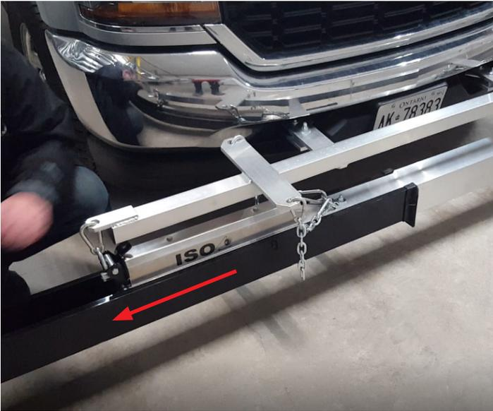
4. Slide the Quick Clean Off Sleeve off of the magnet
