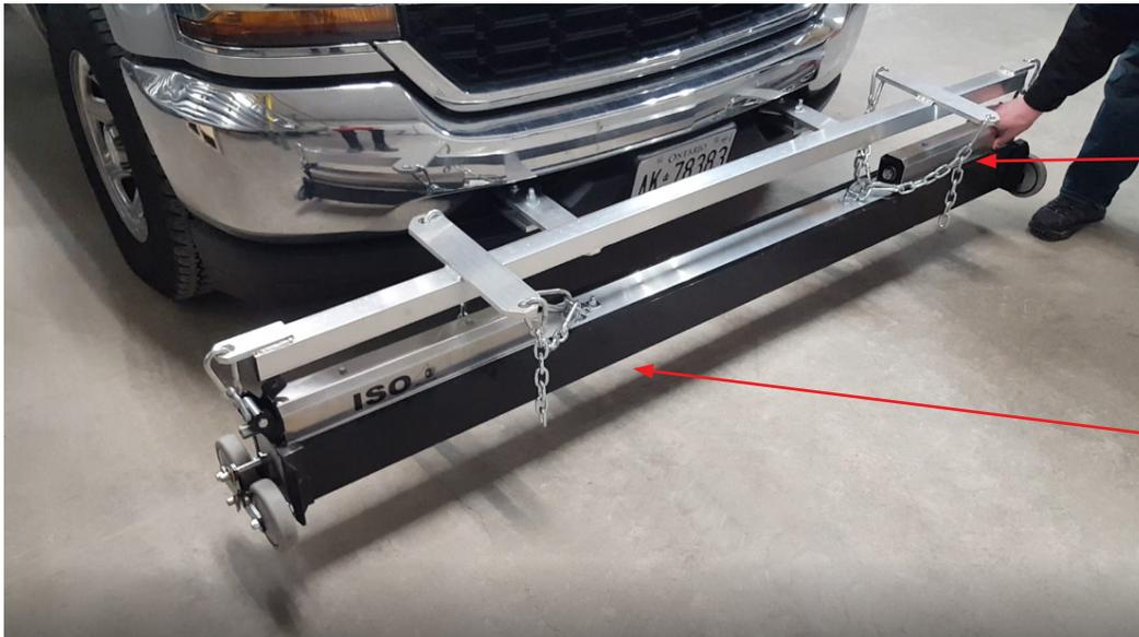
The ISO raised and ready for high speed travel. The hanging chains may be loose but keep them in place for safety. The Adjuster Straps however will be tight and secure.
