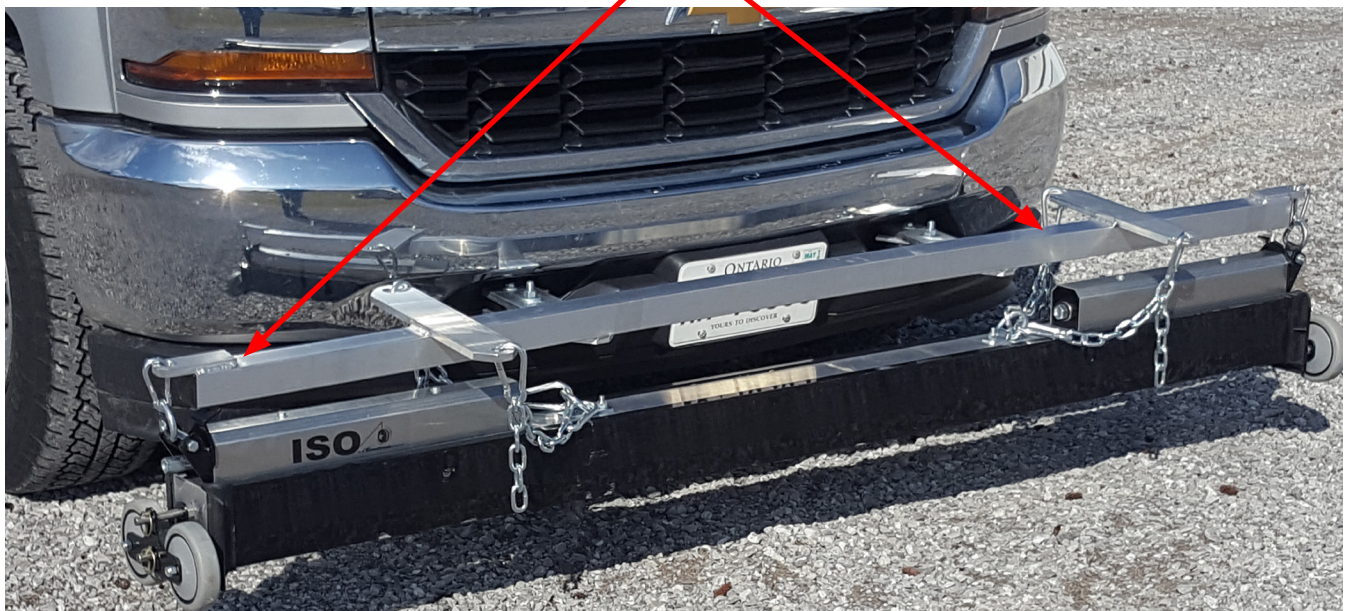
Example custom suspension mounting bracket
