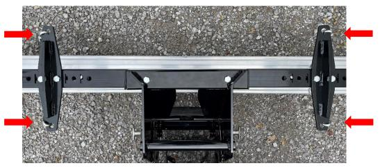
Tip #2: Suspend the Sweeper with the chains all positioned so they are on the outside of the Steel Mounting Plates as shown above.
