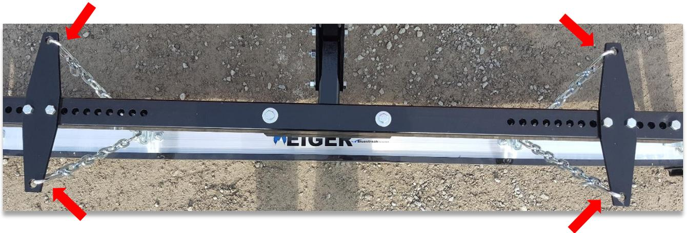
**Tip #2:** Suspend the Sweeper with the Chains all positioned so they are on the inside of the Steel Mounting Plates as shown above.
