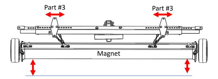
**Tip #3:** The Ground Clearance can be fine tuned by changing the locations of the Steel Mounting Plates (Part #3) inward or outwards, to ensure your magnet is perfectly level with the ground. It is also possible your vehicle or receiver hitch (if used) may not be perfectly level in all directions.
