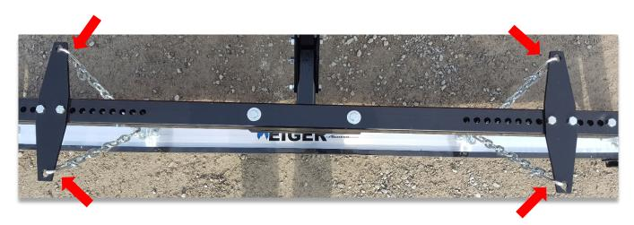
**Tip #2:** Suspend the Sweeper with the Chains all positioned so they are on the inside of the Steel Mounting Plates as shown above.
