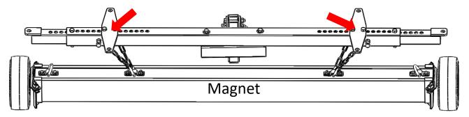
All Magnets should primarily be suspended with 4 chains from the Steel Mounting Plates (Part #3) as shown above. Wheeled sweepers are typically recommended to have the wheels set up ½" off of the ground, and non wheeled sweepers should always be kept as close to the ground as possible without hitting the ground when moving.
