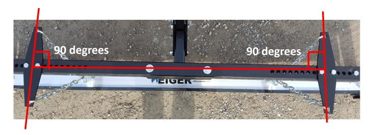
Tip #1: If your magnet appears to be hanging crooked it is possible the Steel Mounting Plates have not been assembled perfectly square. To correct this simply loosen both bolts in each of the 2 Steel Mounting Plates and the problem will correct itself. Retighten the bolts previously loosened.
