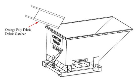
D. Roll up and reinsert Poly Fabric Debris Catchers into Holding Pockets and push all 3 Release Handles down to bottom position.
