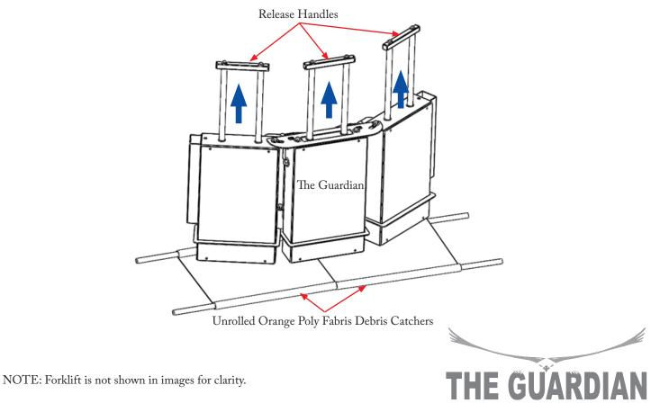
C. Pickup the Poly Fabric Debris Catchers one at a time and dispose of the collected metal debris into appropriate scrap/ swarf/garbage bin.
