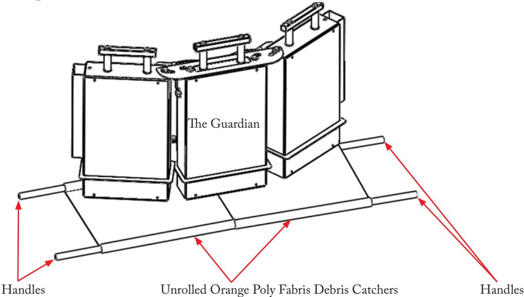
C. Pull upwards on each of the 3 Release Handles until they contact the internal upward stopper. The upward stopper will hold the magnets in the up position. The debris will fall off the bottom of the magnet onto the debris catchers.
