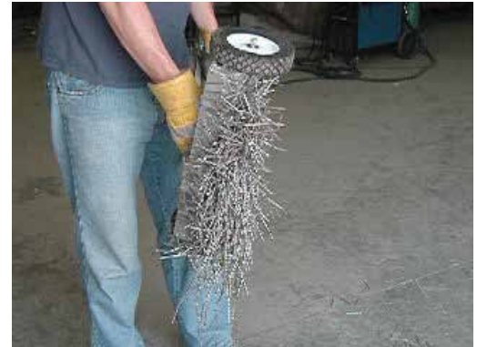
Plenty of pick up power -two layers of permanently charged magnets
