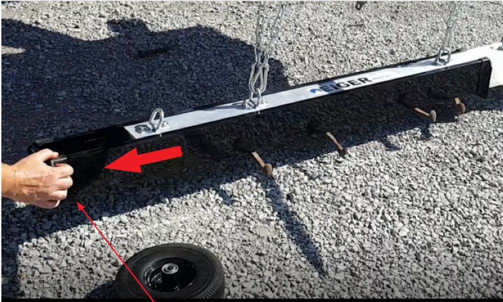
Pull on the Flange on the end of the Quick Clean off Sleeve and pull the Sleeve off.
