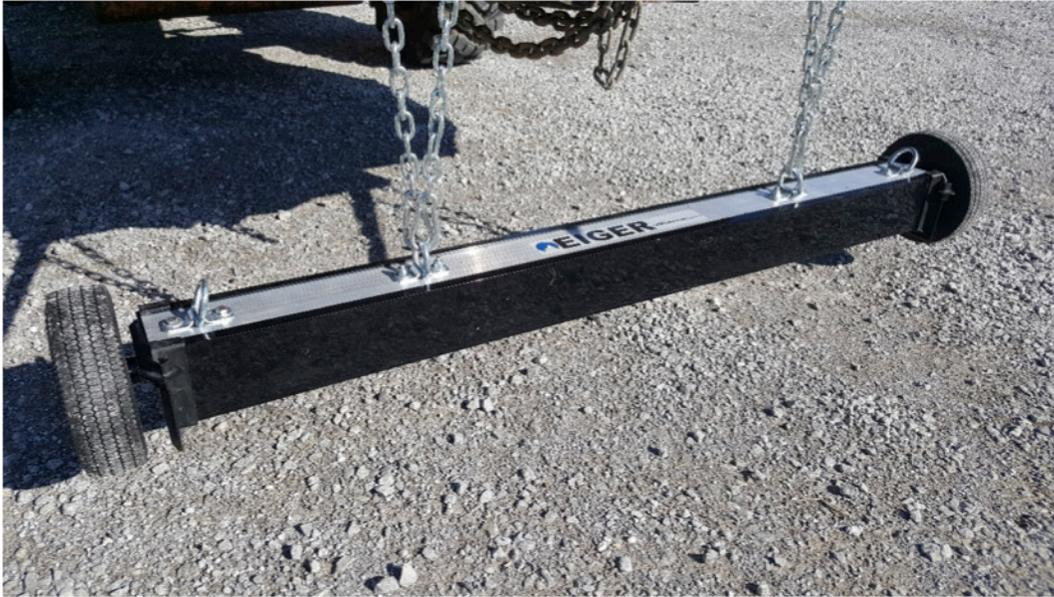
Reinstall the previously removed PVC Quick Clean Off Sleeve, Wheel, Wheel Clip and Sleeve Retainer Clip.
