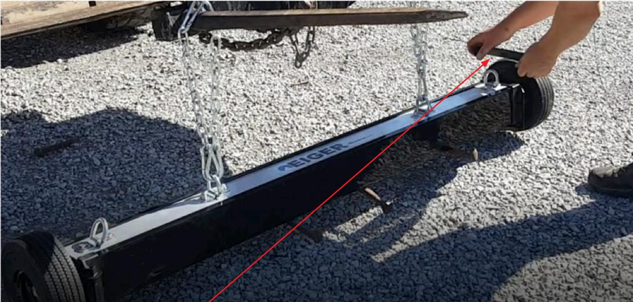
When it's time to clean the magnet off remove the Sleeve Retainer Clip from the opposite end that you want to discharge the metal debris from.
