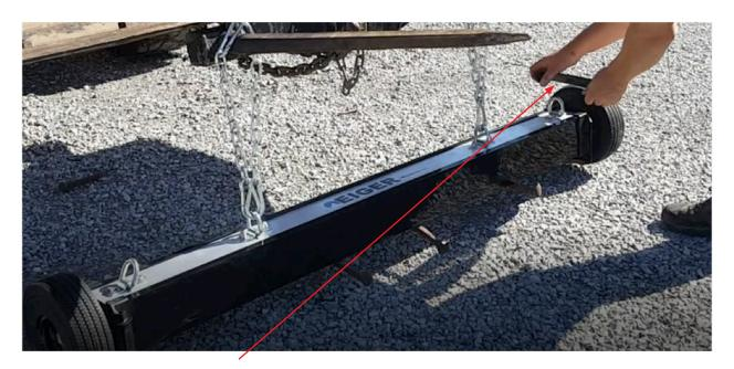
When it's time to clean the magnet off remove the Sleeve Retainer Clip from the opposite end that you want to discharge the metal debris from.
