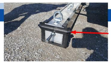
With the magnetic sweeper now suspended from the vehicle using the hanging chains, Re-Install the black PVC Quick Clean Off Sleeve and replace the black PVC quick clean off sleeve retaining Clip on the end of the Sleeve (the black PVC quick clean off sleeve clip is Part F from the cardboard box)
