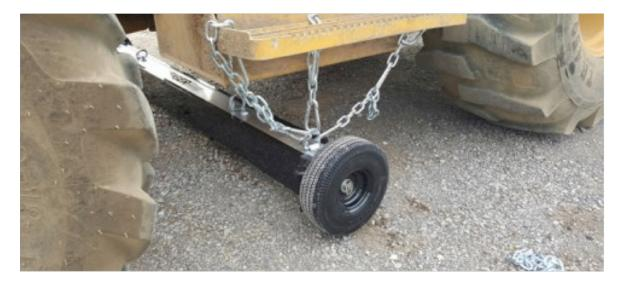
The picture above shows multiple chains in multiple directions to further stabilize the magnetic sweeper to prevent excessive swinging if necessary.
