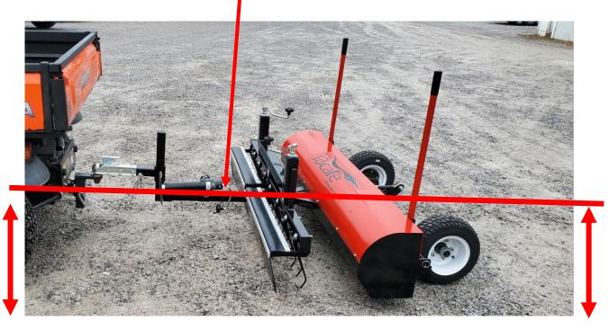
Connect your sweeper with already installed Debris Digging Rake XL with Stoneguard to your tow vehicle.
