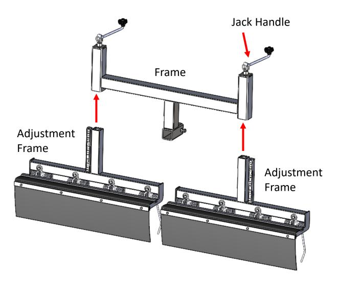
Insert the 2x Adjustment Frames into the Frame, and begin turning the Jack Handle until thread catches and draws them in. Keep turning handle until frames are at top position.
