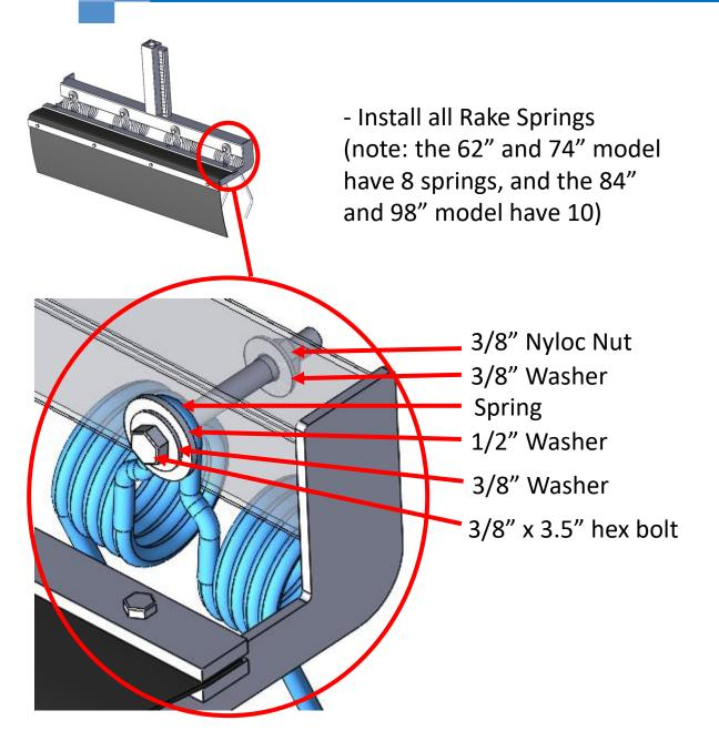
Install a 3/8" x 3.5" hex bolt through a 3/8" washer, through a ½" washer, through a spring, through the steel tube, through a 3/8" washer and finally install a 3/8" nyloc nut. Tighten firmly. Repeat for all springs.
