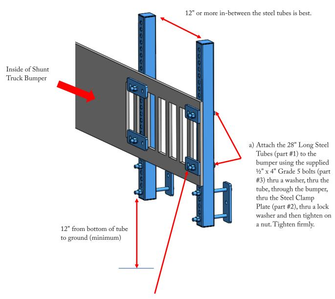
Part #2 - acts as a clamp on the inside of the bumper slot. Place horizontally as shown.
