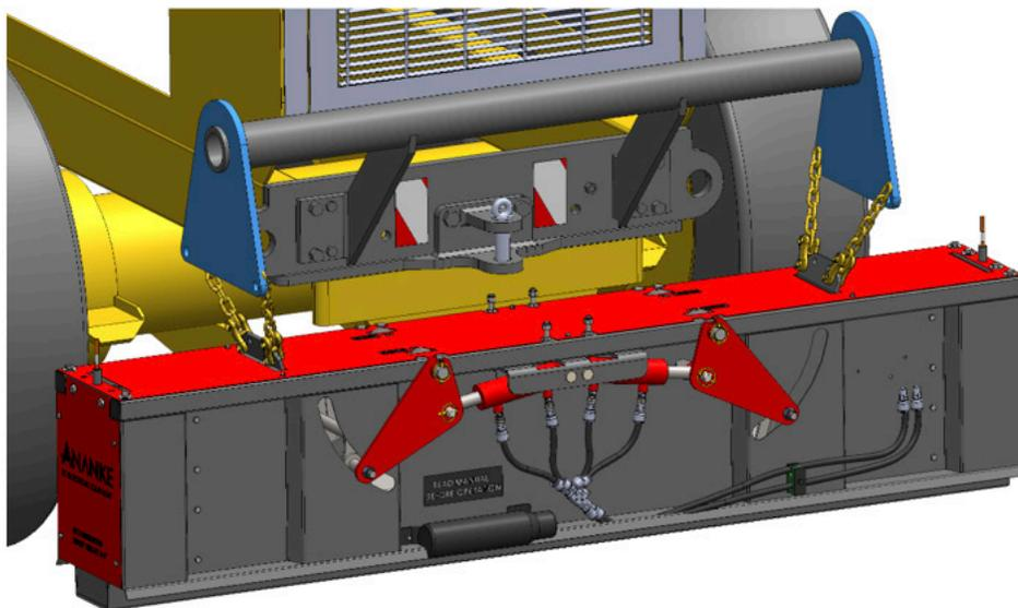
Example 2: Custom fabricated bash bar with steel plates added on the ends to allow chain to be attached and removed as needed. In this example, the bash bar is also removable. Quick links or other hardware would be required to mount the chain to the steel plates.
