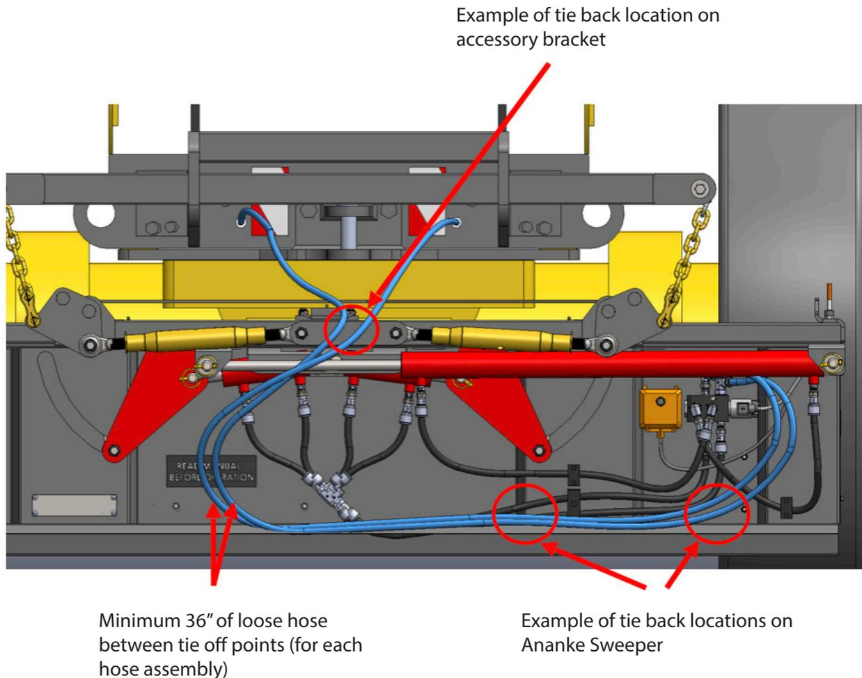
You will need to secure the hose coming off the flow diverter valve to prevent the hose from touching the ground. You may drill holes in the stainless steel flange on the bottom of the sweeper to tie back the loose hose if needed. It is best that all tie off points are not overly tight; they just need to support the hose and allow for some small movement when the side shift bracket is cycled.
