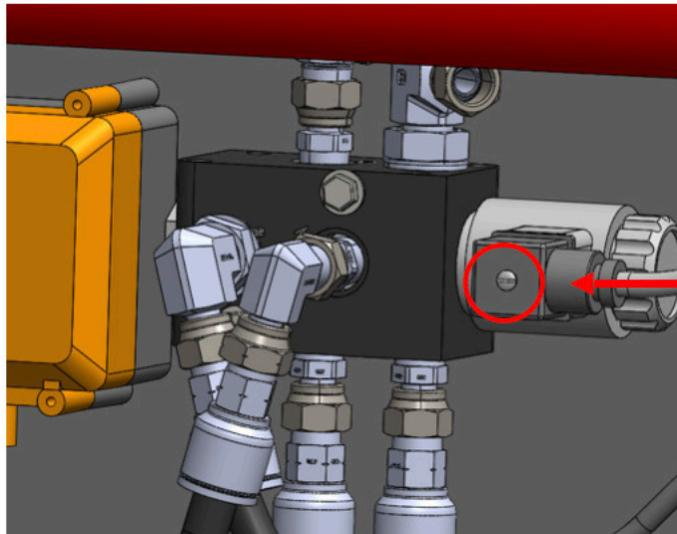
Tighten screw fully. Do not overtighten.
