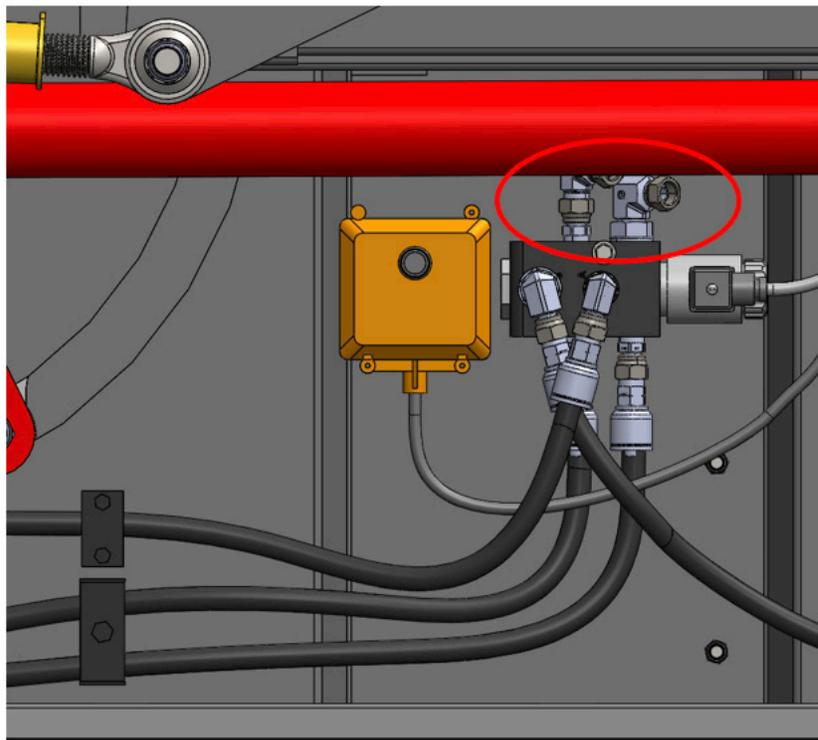
When connecting male NPT ends, ensure Teflon tape or other sealant tape is used to prevent leaks. When it comes time to operate the attachment, if the in-cab controls are providing operation which is opposite from what is expected, the two lines from the motor grader to the flow diverter valve can be swapped. This is easily done at the auxiliary connections on the prime mover.
