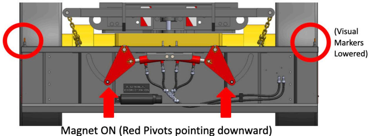
When it is time to clean off the magnet, the in-cab controls for the auxiliary hydraulic circuit will be used. Using the in-cab button or joystick slowly actuate the hydraulics to raise the magnet.
