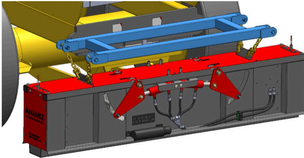
Example 1: Universal Hanging Bracket with some fabricated steel parts to allow mounting to the rear chassis of a motor grader. The bracket is fixed in place and the sweeper is only removable by loosening the bolts on the hanging bracket. Refer to the accessories part of this manual for more information regarding the Universal Hanging Bracket.
