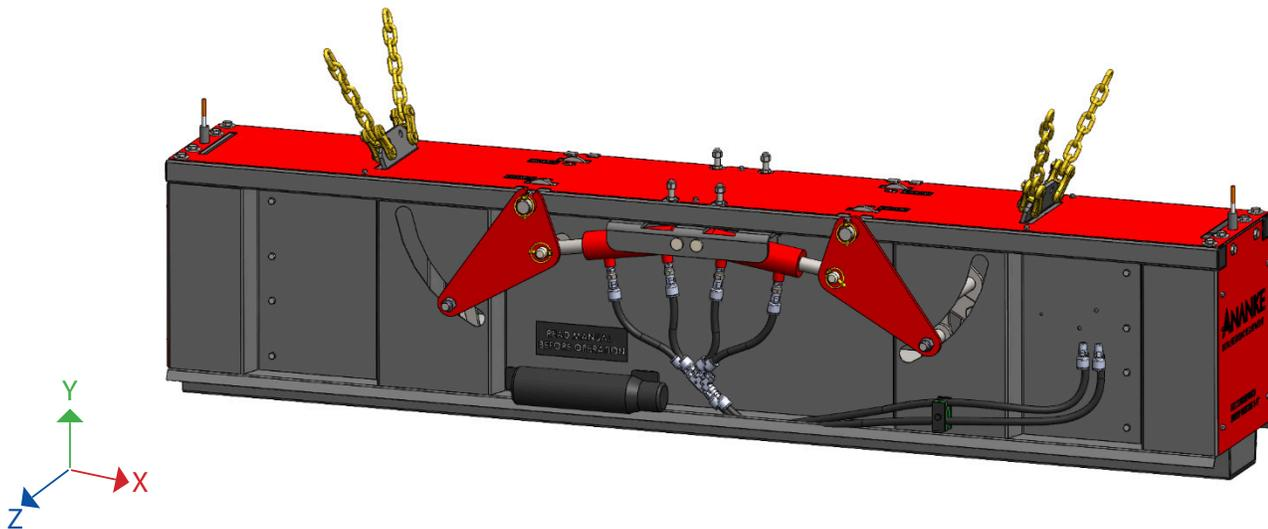
Configuration A: The magnetic sweeper will use a set of hanging plates spaced 59.25 inches apart from each other and hang from transport chain and a twin clevis. Each chain is on an angle outward away from the center of the sweeper in all directions.
