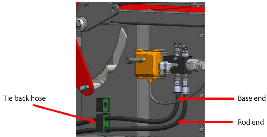
Undo the 6ORB port plugs on the rod end of the cylinder using a hex wrench. Install 2pcs 6ORB to 3/8" NPT swivel fittings into the open ports of the side shift cylinder. Note: PTFE tape should not be used on the ORB connections.
