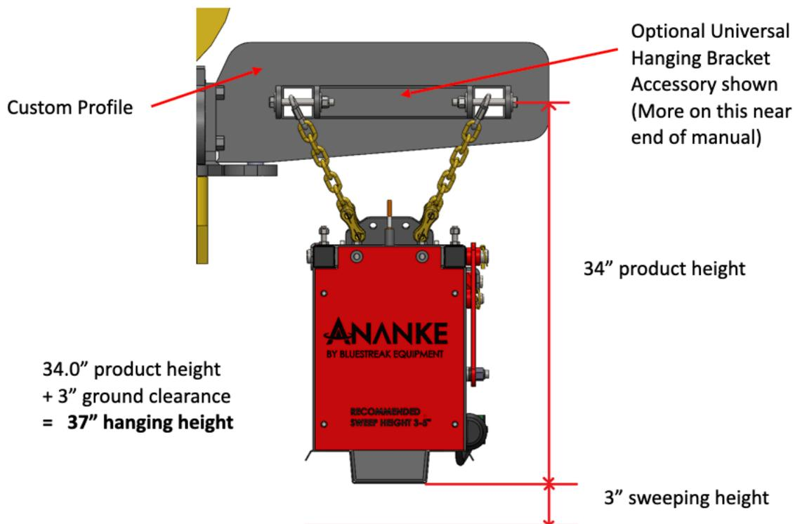
Once a bracket system is fabricated or the Universal Hanging Bracket is modified, you will want to double check the measurements from the ground to confirm it will sit as desired.
