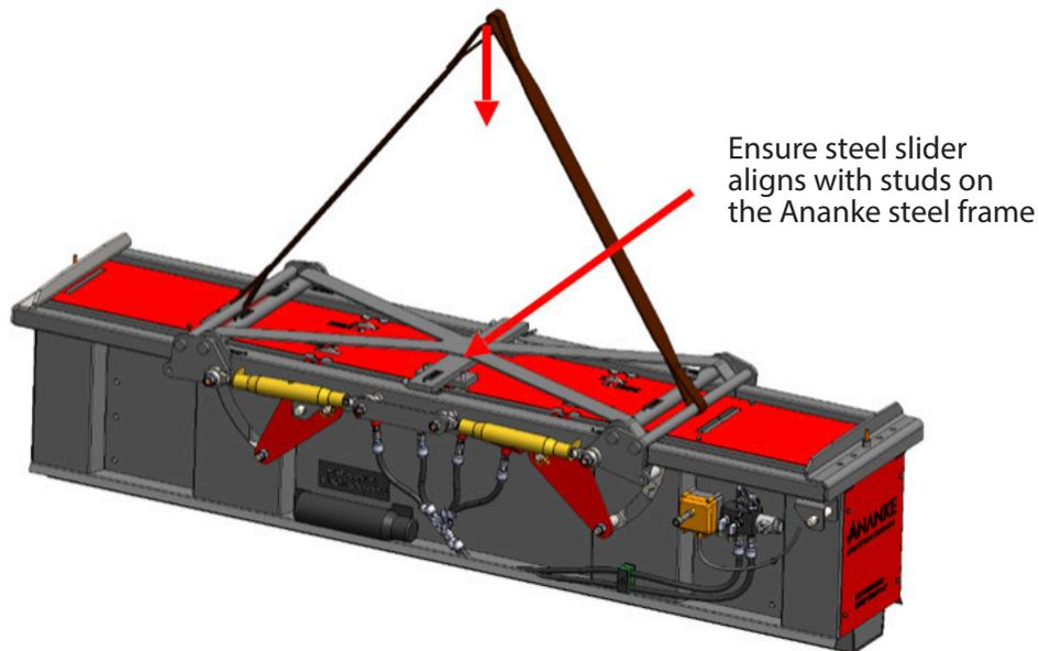
Place 8pcs 0.5" x 3.5" hex bolts into the ends of the sweeper to secure the side shift bracket to the Ananke sweeper frame. Tighten these bolts fully once they are all started. If one or more of the washers are out of position, use a small screwdriver through the center to re-align the washers with the holes of the side shift bracket.
