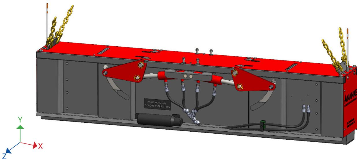
Configuration B: The magnetic sweeper will use a set of hanging plates spaced 92.625 inches apart from each other and hang from transport chain and a twin clevis. The chains point inward (xy plane) and outward (yz plane) from the center of the sweeper so that they do not extend outside the limits of the sweeper.
