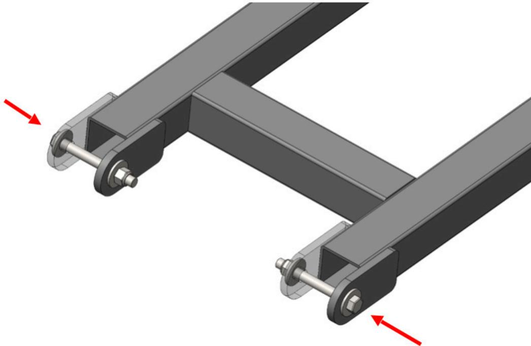
Place a washer over the 5/8" x 5.500" long hex bolt and insert it from the outside of the frame inward. Place another washer on the inside face and secure the bolt in place using the 5/8" nyloc nut. Repeat this procedure for all four corners.
