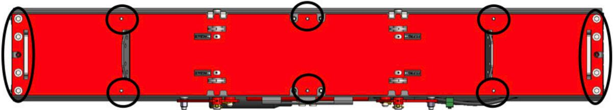
Remove the Ananke sweeper lid by removing the 6pcs  $\frac{1}{4}$ " flange bolts and 6 or 8pcs (depending on configuration)  $\frac{1}{2}$ " x 2.5"L bolts on the top lid. Set the bolts aside for re-installation later.
