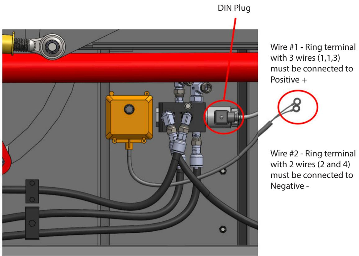
Additionally, the DIN plug must be connected to the diverter valve if it is not already done from factory.
