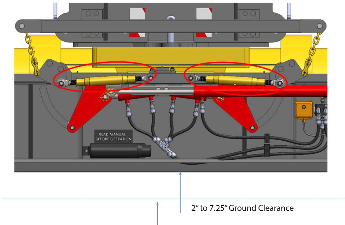
With the side shift bracket attached to the Ananke Magnetic Sweeper there is up to 5.25\" of height adjustment. There is a top link for controlled height adjustment on each side of the Ananke magnetic sweeper. To adjust the height, follow the steps below.
