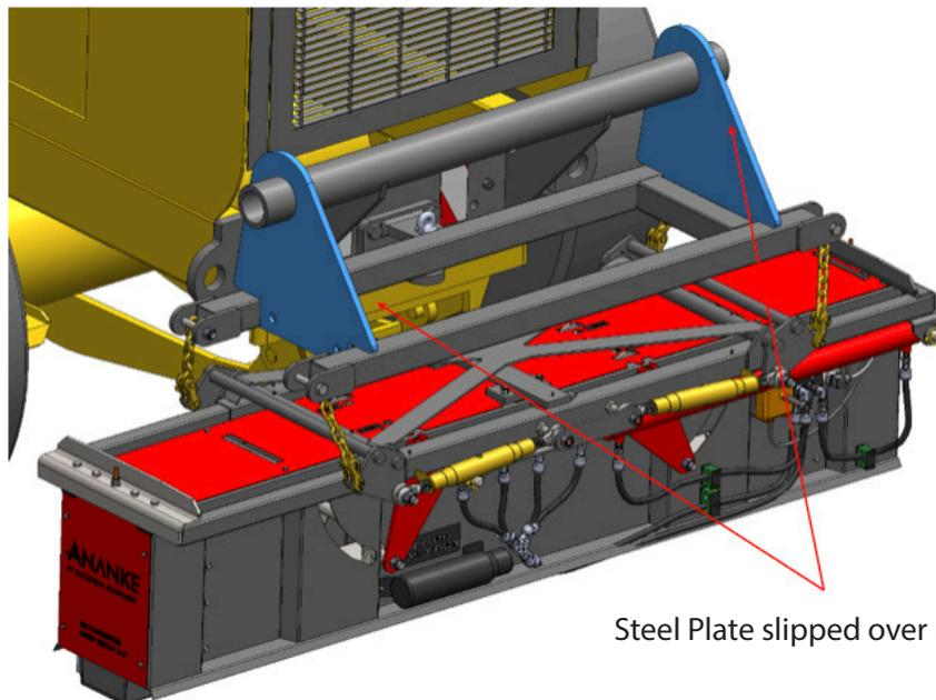
Steel Plate slipped over rear bash bar
