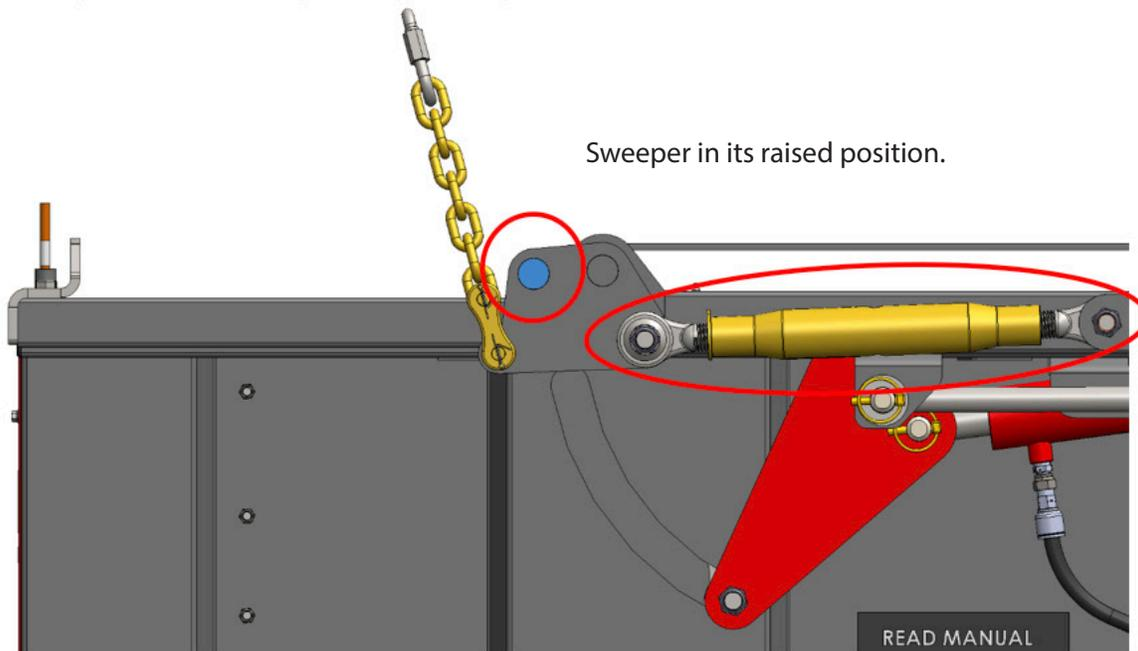
When raising the sweeper, threading in the top link will raise the sweeper. The steel brace of the pivot (shown in blue) will bottom out on the side shift bracket when it is in a fully raised position. There are still threads exposed on the top link however do not try and force it past this position.
