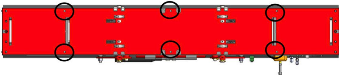
Place stacks of 2 washers on top of the lid over each of the open holes on the ends of the sweeper. There should be 8pcs on each side of the sweeper
