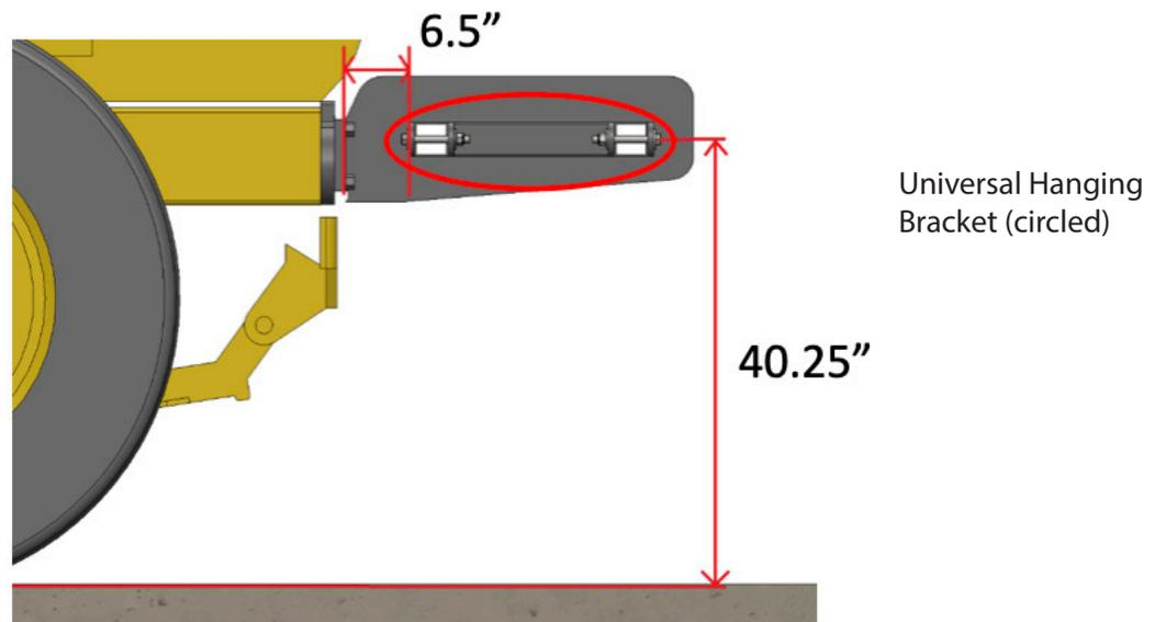
The center of the bolts on the hanging bracket should be 40.25" off the ground when used in combination with the side shift bracket. The bracket should not be closer than 6.5" to the back of the prime mover.
