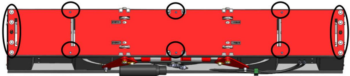
Remove the 6pcs 1/4" flange bolts on the top of the sweeper and the 8pcs 1/2" hex bolts with washers to remove the red lid. Set the hardware and the lid aside.
