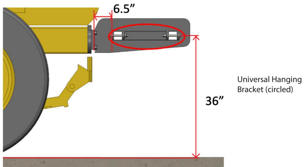
The center of the bolts on the hanging bracket should be 36" off the ground for use with the Ananke sweeper (without side shift bracket). The bracket should not be closer than 6.5" to the back of the prime mover.
