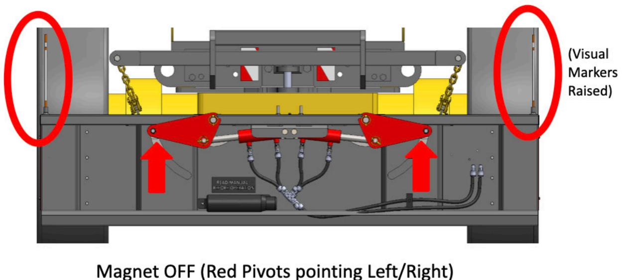
Once the Ananke is in a raised position the collected debris will fall to the ground beneath the magnet surface. Verify that the visual markers can be seen during normal operation, and if they can't, they may need to be extended in length.
