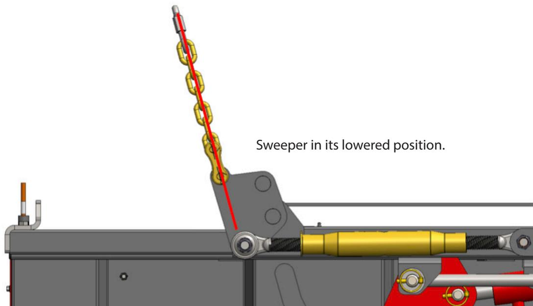
When lowering the sweeper, unthreading the top link will lower the sweeper. The position illustrated above shows the chain parallel to the bottom of the pivot. Unthreading the top link past this position will not provide any more height adjustment for the sweeper. Do not try and extend it past this position as this will only raise the sweeper.
