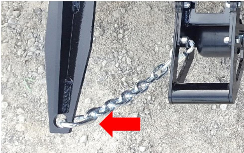
Connect the upper end of the chain as shown, so it is on the inside of the upper connection points.
