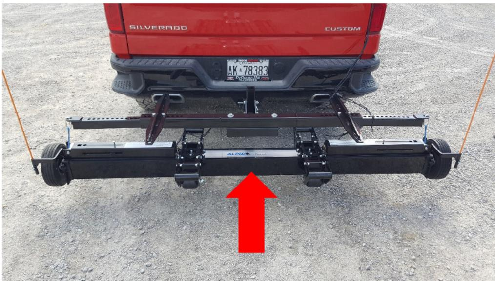
Press the up button on the remote and lift the sweeper until it is an inch or so from contacting anything above it.
