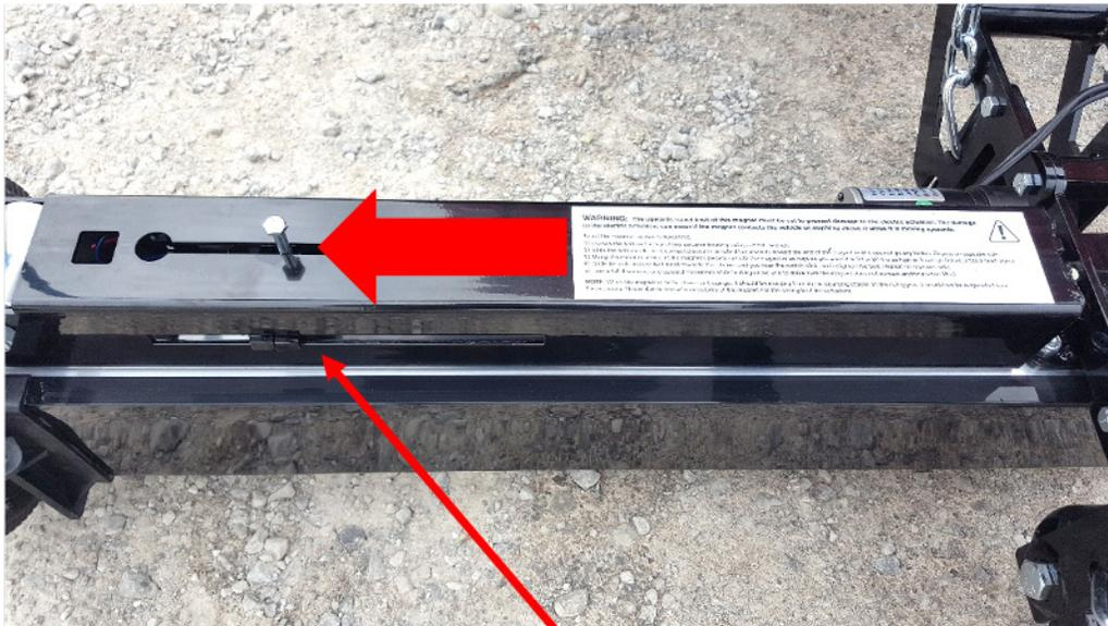
Slide the limit contact block outwards until it contacts the other contact block. Repeat for opposite side.
