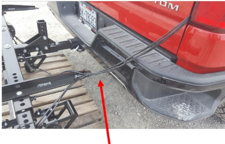
Route the Wires and Connect to a 12v Battery source on your vehicle.
