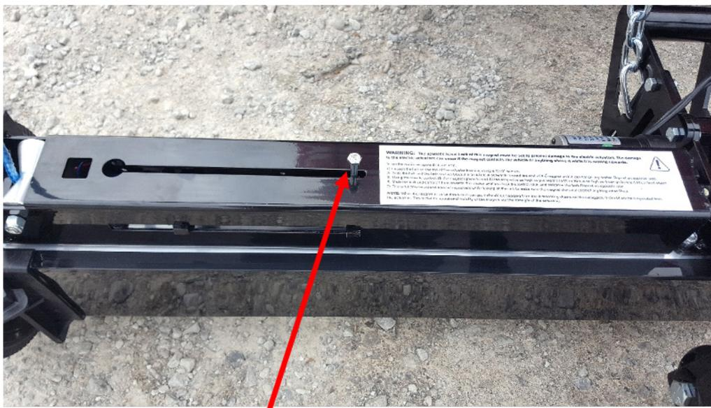
Loosen the Bolt in the top of each Actuator using a 7/16" wrench.
