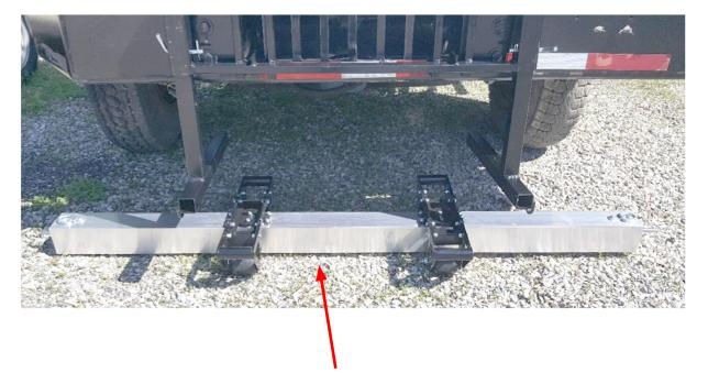
Set the Aether underneath your vehicle in preparation for mounting
