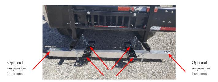
Suspend the sweeper from the 4 mandatory suspension holes using the chains and quick clips provided. The target height between the bottom of the magnet and the ground is 3 1/8" (with the quick clean off sleeve removed).
