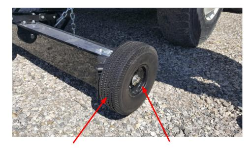
Install the 10" flat proof wheel on the wheel bolt. And insert the lynch pin. Do the same on the other end. Assembly and installation is now complete. The wheels of the Aether should be approximately ½" inch off the ground.
