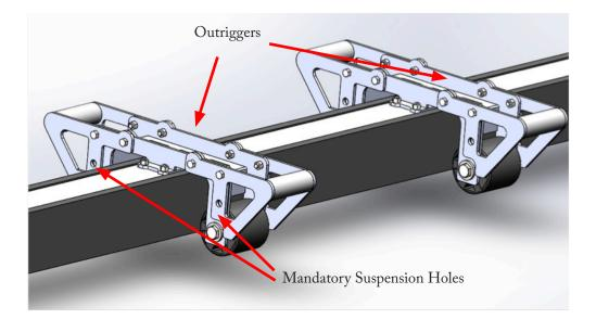
The 2 holes on the outside of each outrigger are the MANDATORY suspension locations where the chains (quick clips) need to be connected to the sweeper.
