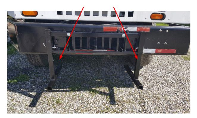
Example of custom suspension mounting bracket built for an Ottawa shunt truck.
