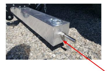
Thread in 1 wheel bolt on each end of the Aether magnetic sweeper aluminum end cap. Then tighten the wheel bolt using a 7/8" wrench.
