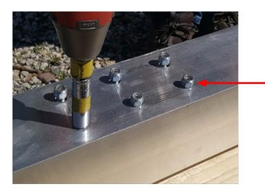
Now remove the 12 nuts (6 per outrigger installation location) from the top of the sweeper using a 9/16" socket.
