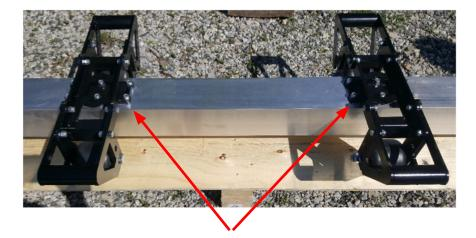
The install both of the outriggers and re-install and tighten all 12 previously removed nuts firmly with a 9/16" socket.
