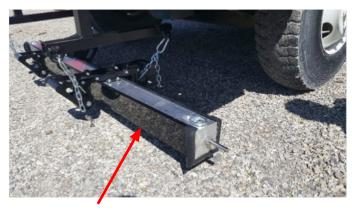
Slide the quick clean off sleeve over top of the aluminum housing.
