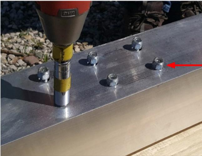
Now remove the 12 nuts (6 per outrigger installation location) from the top of the sweeper using a 9/16" socket.
