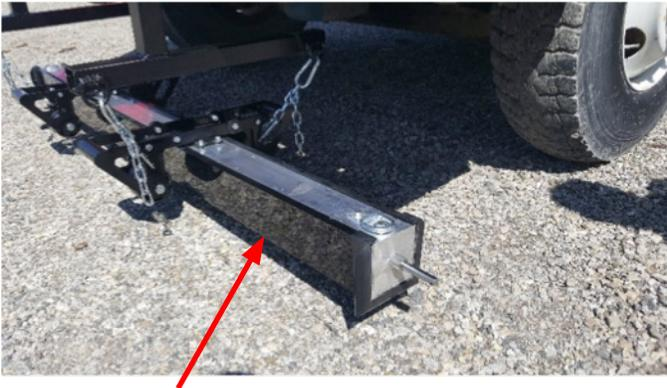
Slide the quick clean off sleeve over top of the aluminum housing.
