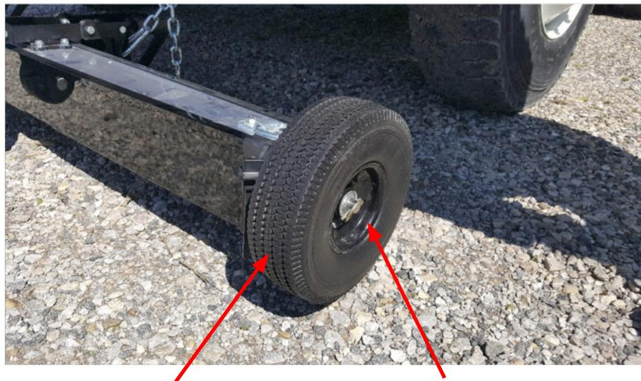
Install the 10" flat proof wheel on the wheel bolt. And insert the lynch pin. Do the same on the other end. **Assembly and installation is now complete.** The wheels of the Aether should be approximately ½" inch off the ground.
