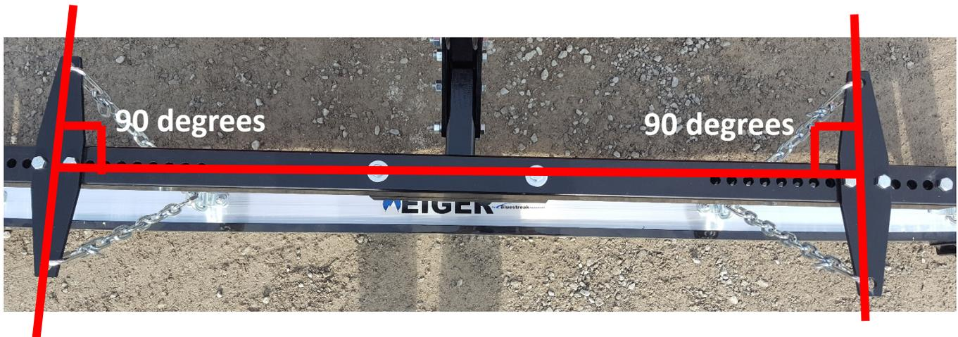
**Tip #1:** If your magnet appears to be hanging crooked it is possible the Steel Mounting Plates have not been assembled perfectly square. To correct this simply loosen both bolts in each of the 2 Steel Mounting Plates and the problem will correct itself. Retighten the bolts previously loosened.
