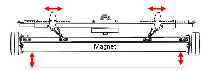
**Tip #3:** The Ground Clearance can be fine tuned by changing the locations of the Steel Mounting Plates inward or outwards, to ensure your magnet is perfectly level with the ground. It is possible your vehicle or receiver hitch (if used) may not be perfectly level in all directions.
