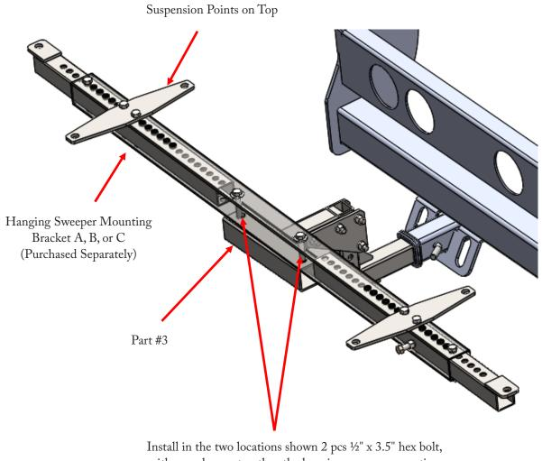
with a washer on top thru the hanging sweeper mounting bracket, thru the top of Part #3 and install a lock washer and nut inside Part #3.
