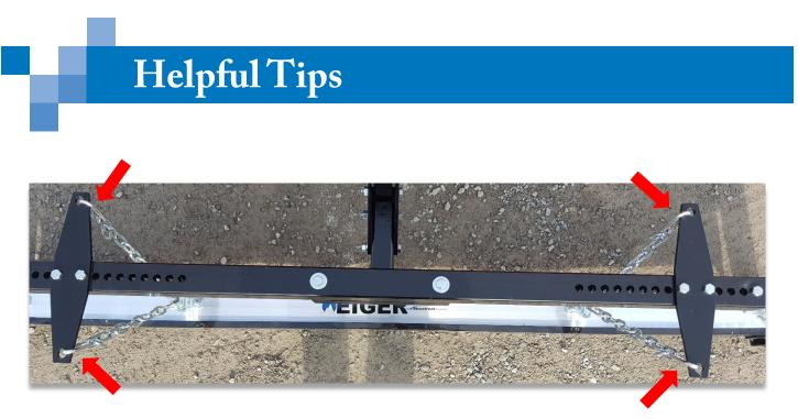
Tip #2: Suspend the Sweeper with the Chains all positioned so they are on the inside of the Steel Mounting Plates as shown above.
