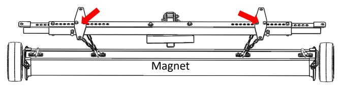
All Magnets should primarily be suspended with 4 chains from the Steel Mounting Plates as shown above. Wheeled sweepers are typically recommended to have the wheels set up ½" off of the ground, and non wheeled sweepers should always be kept as close to the ground as possible without hitting the ground when moving.
